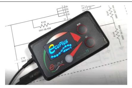
EcuPlus<sup>®</sup> Easy **Counter T3**, is a highly evolved tachometer. It allows to measure the engine revolutions, the temperature, the elapsed time, the maximum values of the measured during the test and send them to the smartphone.
