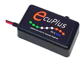
EcuPlus® TC-I **Easy** is a timing control unit compatible with TCI-IKEDA Ignition Systems with two magnets 60, 70 and 89 mm of diameter.
