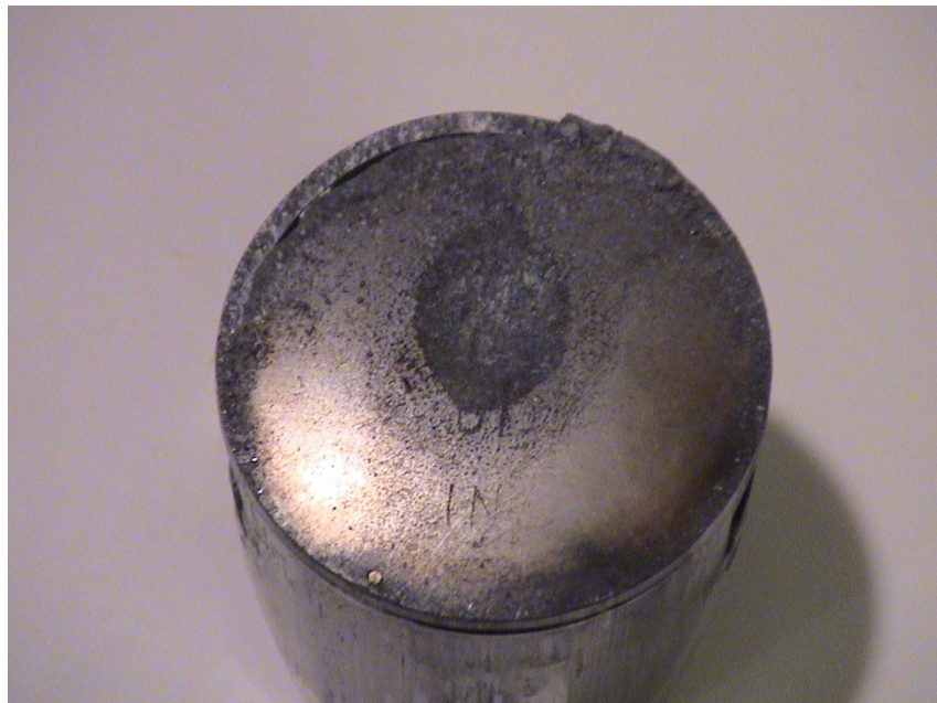
Picture 3: Lean carburetion and premature combustion
