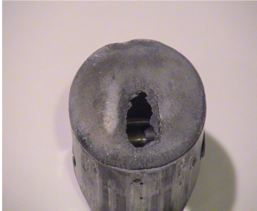
Picture 2: Detonation from lean mixture
