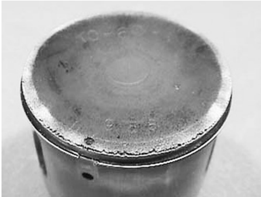
Picture 5: Detonation caused by compression
